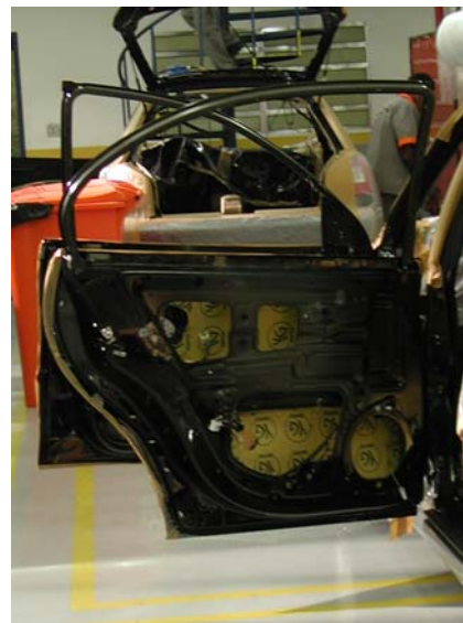
Figure 7. YellowGard® installed inside a door.
